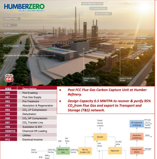
FCC Flue Gas Carbon Capture Unit
